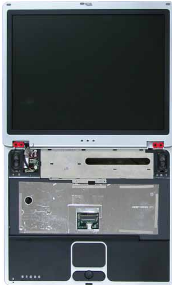
Fig. 24 Removing screws retaining LCD Module
